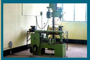
The workshop under Triguna Sen School of Technology contains highly sophisticated machines presenting a unique and unparalleled quality. These include Machine Shop, Welding, Fitting, Smithy and Carpentry Shops. The workshop has also Centre Lathes, Turret Lathe, Drilling Machines (sensitive, polar & radial), and Slotting Machine, Grinder Pedestal, Surface Grinder M/C and many other machines.
